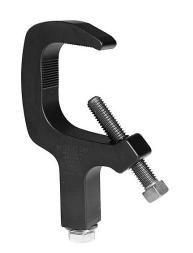
The Mega-Clamp is the world's new standard theatrical lighting C-Clamp. The Mega-Clamp is created from high tensile, aircraft grade, extruded aluminum, so it's both stronger and lighter than cast iron damps. The Mega-Clamp's safety factor far exceeds industry standards, breaking at over 2-1/2 tons at an independant testing laboratory. It is half the weight, and twice as strong as most cast iron damps.
