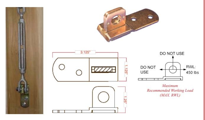
Made from heavy-gauge steel and pre-drilled for assembly with two 1/4" bolts. This smaller version of the 90-degree Shackle Plate™ will mount easily and more discreetly into the side-stiles of any wood or metal flat. 1/2" opening for hardware attachment.
