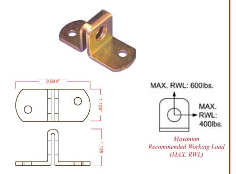
Made from heavy-gauge steel and pre-drilled for assembly with two 1/4" bolts. Smaller version of the Shackle Plate<sup>™</sup> that will mount easily and more discreetly into the bottomrail of any wood or metal flat. 1/2" opening for hardware attachment.
