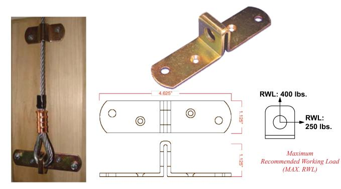
Made from heavy-gauge steel and pre-drilled for assembly with two 1/4" bolts and two #8 or #10 flat head screws. 1/2" opening for hardware attachment.
