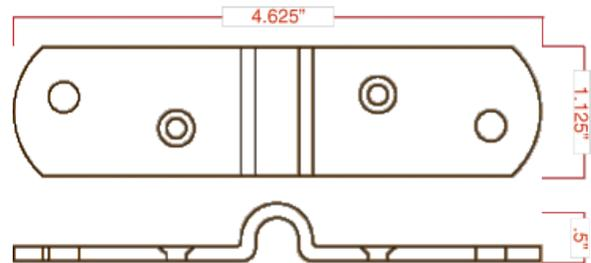
Made from heavy-gauge steel and pre-drilled for assembly with two 1/4" bolts and two #8 or #10 flat head screws.
