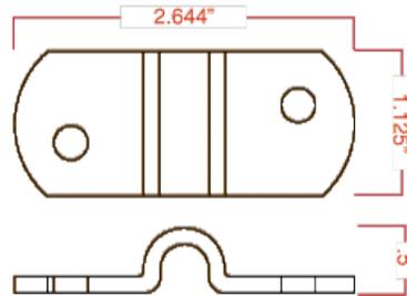
Made from heavy-gauge steel and pre-drilled for assembly with two 1/4" bolts.
