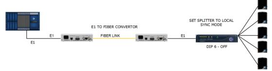
The antenna connections are switched between RJ45 and Fiber routing using dip switches set inside the splitter.
