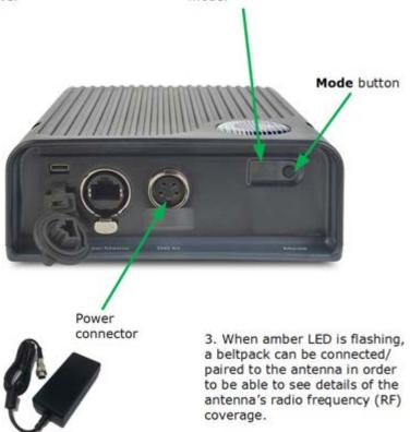
1) Connect power to the antenna and at the same time press the black Mode button on the base of the antenna. This puts the antenna in standalone mode, and opens it for pairing to a beltpack.
