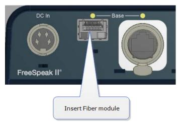
Once the modules are installed, the Base Station and the splitter can be cabled with the correct Fiber cable (single mode or multi-mode depending on existing cabling). You will see the Base Connection indicator on the front of the splitter change from RJ45 to Fiber.
