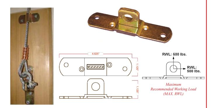
Made from heavy-gauge steel and pre-drilled for assembly with two 1/4" bolts and two #8 or #10 flat head screws. 1/2" opening for hardware attachment.
